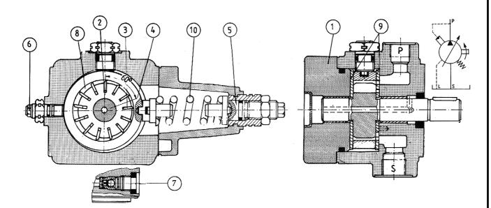
Hydraulic pumps type V3 are vane pumps with variable displacement and pressure control. Pumps type V3/12 are composed of a housing 1, rotor 2 with simple vanes 3, stator 4, pressure regulator 5, volume screw 6, valve for automatic air bleed 7 and control discs 9.
