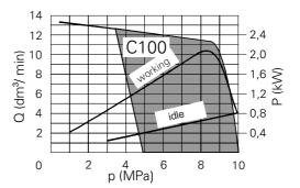
Leakage - operating pressure curve
