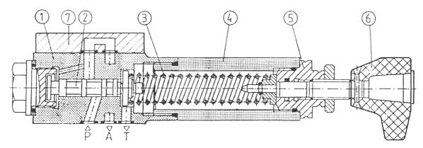
The spool 2 is held in neutral position in the housing 1 by the spring 3. At the same time pressure in line A affects the spool surface opposite the spring. The valve is open in initial position. The spring force is set by turning the hand knob 6 of the setting element 5, which is screwed in the sleeve 4. If pressure exceeds the value set at the spring, the spool moves along and reduces the flow from P to A.
