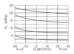
$P_A = f(Q)$  - output pressure in relation to flow rate
