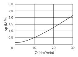
$\ensuremath{\,{}^{\textstyle \square}}\ p$  = f(Q) - pressure drop at check valve in relation to flow rate
