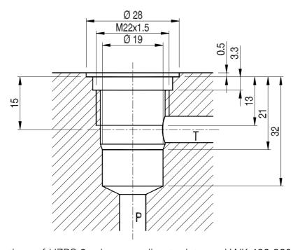
Detailed specifications of UZPS 6 valve according to data card WK 492 860
