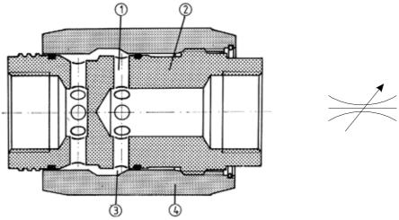
Fluid gets at the throttle point 3 formed between the housing and the adjustable sleeve 4 through side bores 1 in the housing 2. By rotating the sleeve, the circular section at the throttle point may be steplessly changed. The valve throttles in both directions.
