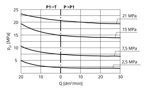
Characteristic curves of minimum pressure drop in relation to flow rate in the direction of flow P - P1
